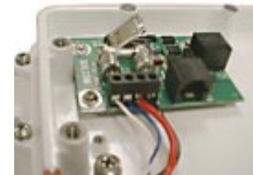
Figure 11. Lift the socket cover
